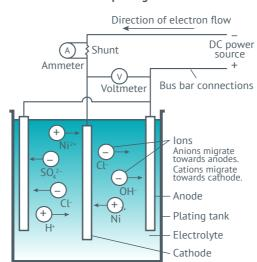
Figure 1 Basic electrical circuit for electroplating
