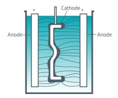
the solution. The complex relationship between these factors and metal distribution is termed the *throwing power*. Throwing power can be determined experimentally. Solutions exhibiting a positive value will be capable of reducing the variation in thickness between prominent and recessed areas. Conversely solutions with negative values, such as chromium plating solutions, may exhibit a greater thickness variation than would be expected based purely on geometric factors.
